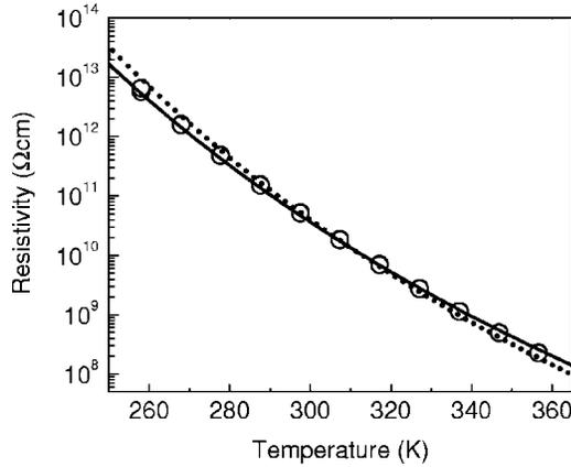
FIG. 4. Illustration of confidence range for  $\rho(T)$  fits. Open circles: experimental data from Fig. 3. Straight line: scenario (i) with 20-meV lower effective ionization energy. Dotted line: theoretical behavior of pure (intrinsic) material.
