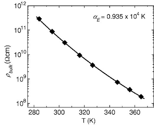
FIG. 10. Temperature dependent bulk resistivity measurement on a SI-CdZnTe test device in the range between 284 and 365 K. The line is a fit according to Eq. (8) yielding  $\alpha_E = 0.935 \times 10^4 \text{ K}$ .
