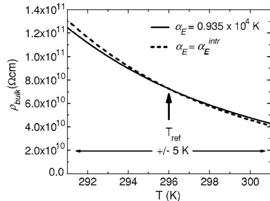
FIG. 11. Comparison of the temperature dependence of the bulk resistivity of the test device from Fig. 10 with the intrinsic slope ( $\alpha_E^{\text{intr}} \sim 1.02 \times 10^4 \text{ K}$ ) in a  $\pm 5 \text{ K}$  temperature window around  $T_{\text{ref}} = 296 \text{ K}$ .
