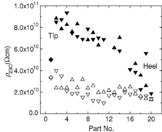
FIG. 14. Tip-to-heel  $23^\circ\text{C}$ -resistivity profile of a  $\text{Cd}_{0.9}\text{Zn}_{0.1}\text{Te}$  ingot measured on devices in the dual  $I$ - $V$  guard electrode configuration (filled triangles) and erroneous data from measurements on devices with a simple parallel plate electrode configuration (open triangles). Two neighboring rows of  $5 \times 5 \times 2$  mm<sup>3</sup> axial parts have been examined for each of the configurations (upside and downside tipped triangles).
