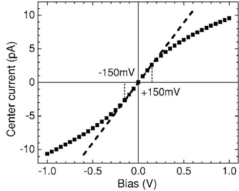
FIG. 6. Current-voltage characteristics measured on the guarded  $5 \times 5 \text{ mm}^2$  center electrode of a 2-mm-thick CdZnTe detector and linear fit in the bulk conductivity limited range (dashed line).
