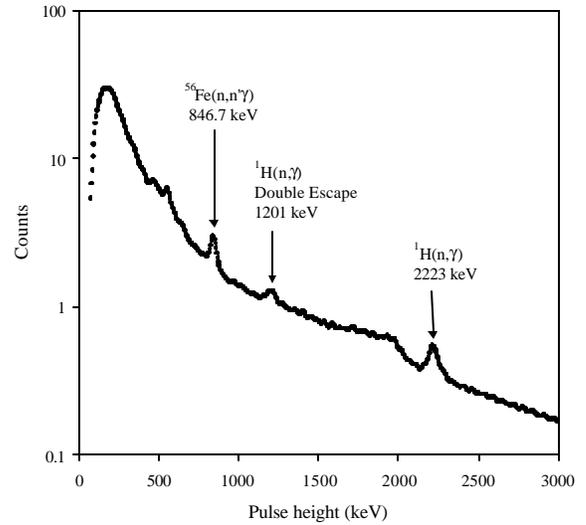
Fig. 2. Gamma ray spectrum measured by an 8-element CdZnTe detector array. The detector array was placed next to <sup>252</sup>Cf source, which was surrounded by a large mass of stainless steel.
