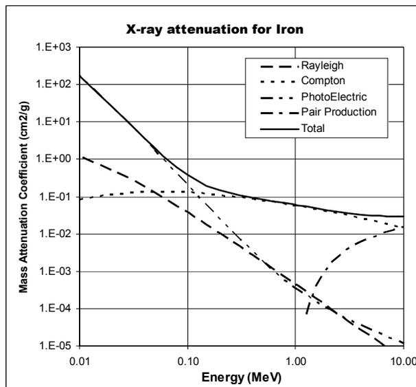
Figure 2. Attenuation coefficients as a function of energy for iron<sup>3</sup>.
