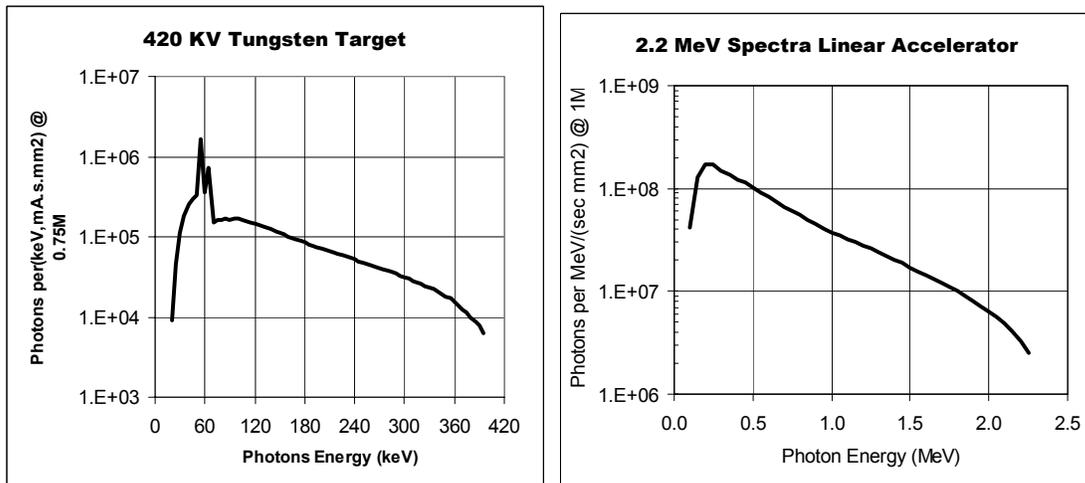
Figure 1: X-ray Spectrum,  $I_0$ , for 420 KeV and 2.2 MeV Bremsstrahlung Sources<sup>1</sup>.
