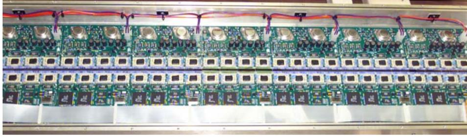
**Figure 7 ARDEC's line scanning, x-ray energy discriminating detector.**
