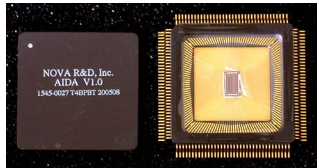
Fig. 2. AIDA layout (top) and photograph of chip in CQFP (bottom).
